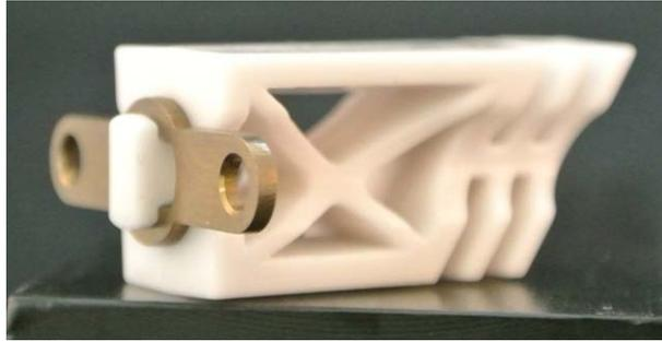
**Figure 1** The biocomposite cage composed of 30% bicalcium phosphate dispersed in amorphous poly L-lactide-co-D,L-lactide polymer accepts either titanium or SS wings that clip onto a T-shaped post and can be rotated 360° to the desired location. The end is tabbed to facilitate cutting the cage to the desired length based on the proximal tibial osteotomy depth.
